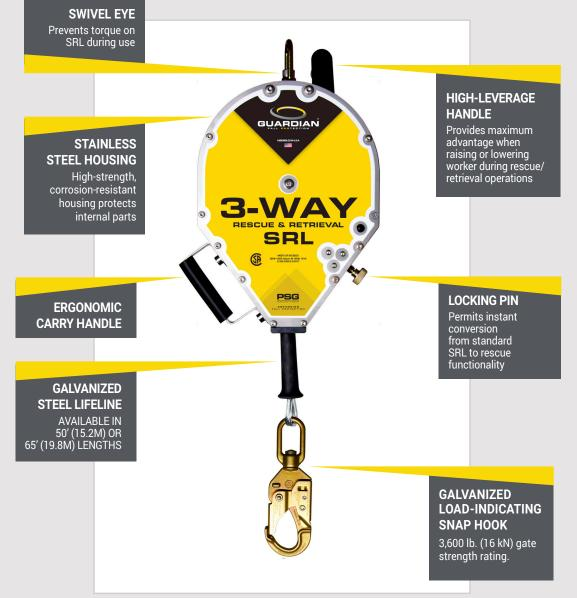
Lifeline: Galvanized Steel Snap Hook: Galvanized Steel Capacity: ANSI: 130-310 lbs. (59-190 kg.); OSHA & CSA: 100-310 lbs. (45-190 kg.)
