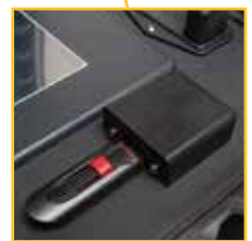
The built-in USB port allows easy connection to a data storage device.
